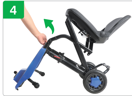
Step 4 Lift the folding lever upwards to fold the body, folding is completed.
